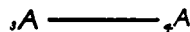
Fig. 3.—If the distance A—A is equal to that between the atoms adsorbed, the activation energy will be high.
